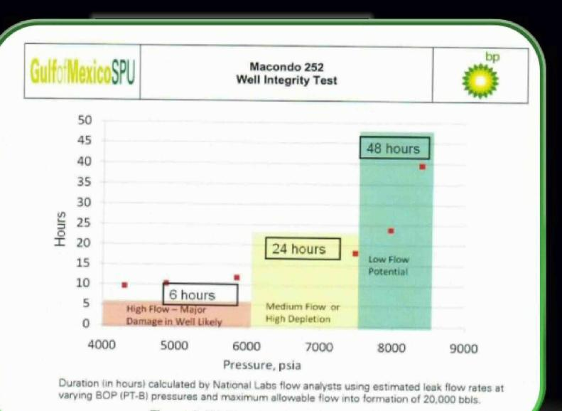
Figure 2: Well Integrity Test Duration Guidance
