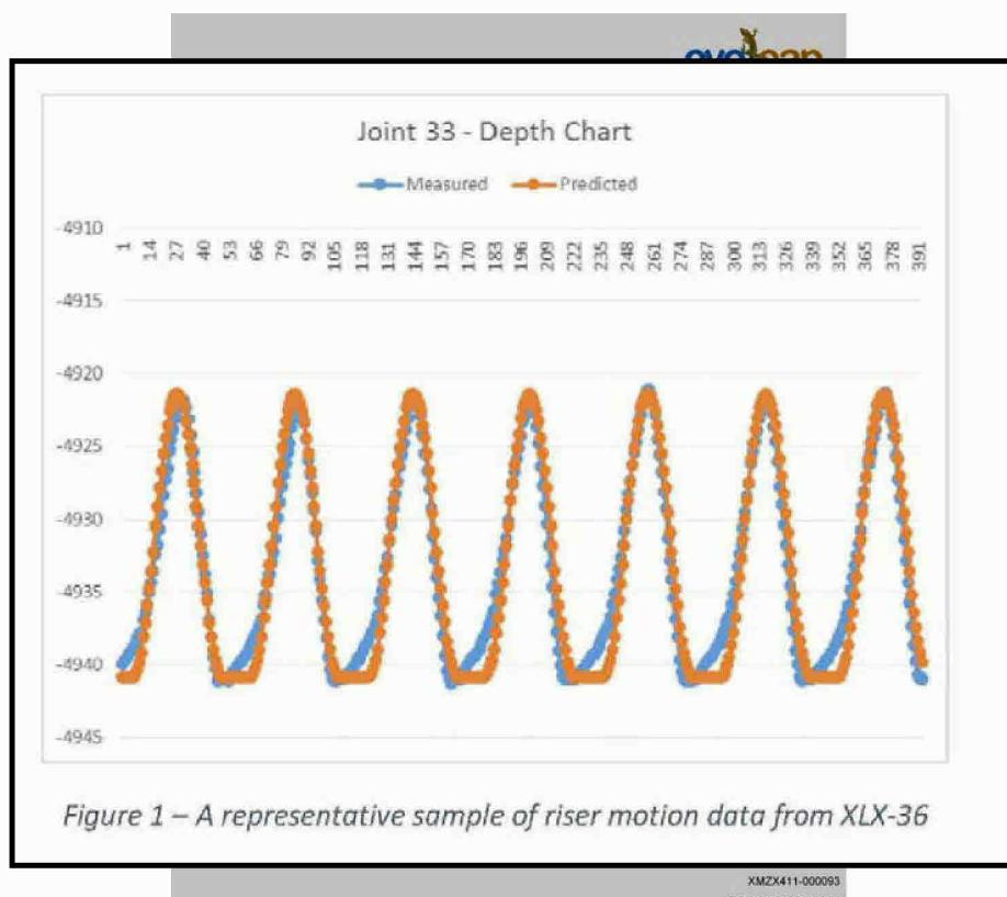
Figure 1 – A representative sample of riser motion data from XLX-36
